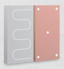
Tap the board back firmly using a straight edge ensuring that the vertical edge is plumb. Fasten to wall with 5 ultra fixings (1 in each corner and 1 in centre).
